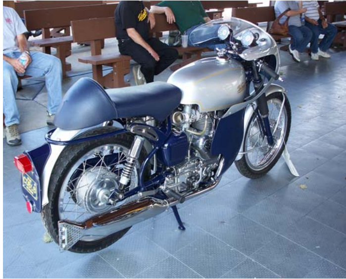
1968 500cc Velocette Venom Thruxton Veeline with Avon racing fairing, owned and ridden by Keith Hogland. Note the huge Amal Concentric carburetor.
