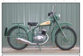
Stock 1949 BSA 125 Bantam, note the pillion rack, rigid rear frame, absence of rear seat and rear foot-pegs.
