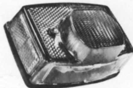
391-56513 Tail Lamp Unit 1973 and later 391-54584930 Lens
