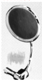
561-05/A & 561-06 HALCYON Classic style barend mirrors with stainless heads; nylon sealing ring, ball cup joint for maximum adjustment; stainless arm & two piece chrome clamp for secure fixing; fits 7/8 or 1" bars. 561-05 econo also available.
