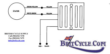
IF YOU HAVE AN OLD **6** VOLT **3** WIRE STATOR YOU CAN CONVERT IT TO **12** VOLT BY JOINING THE GREEN/BLACK AND GREEN/YELLOW WIRES TOGETHER THEN CONNECT THOSE TWO TO ONE OF THE YELLOW AC WIRES AND THEN CONNECT THE GREEN/WHITE WIRE FROM THE STATOR TO THE OTHER YELLOW AC WIRE OF YOUR **SPARX** BOX, THEN THE RED+ AND THE BLACK- CONNECT INTO YOUR MOTORCYCLE WIRING. PLEASE DON'T FORGET TO CHANGE YOUR BATTERY/ BULBS AND HORN ETC TO **12** VOLT AS WELL.
