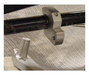
9 Attach the rose joint to the frame bracket using the cap screw, and nut provided.
